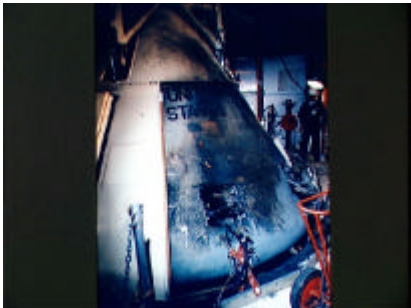
Figure 5: External view of fire damage to Apollo 1 Command Module (NASA S67-21295).
