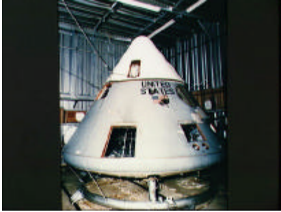
Figure 4: Apollo 1 Command Module after fire (NASA S90-35348).
