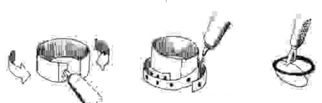
Cut the G-6 stripe and roll it to form a cylinder. The red side is the external one. Glue the G-7 around the G-6 and glue it. Please check if the thickness of this roll correspond to the thickness of the G-8 disk. If not cut a part of it or add another piece obtained using the residual part of the sheet. Cut the G-8 ring.
